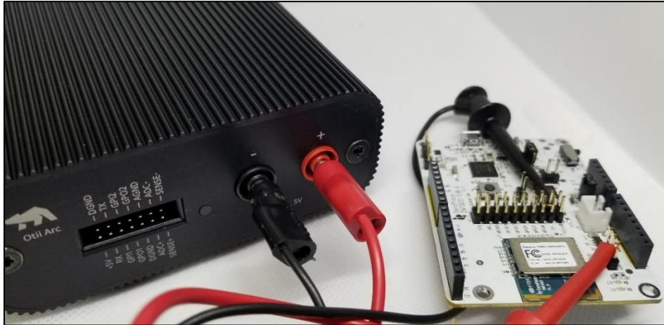
Figure 9: Current measurement setup using Otti Arc
